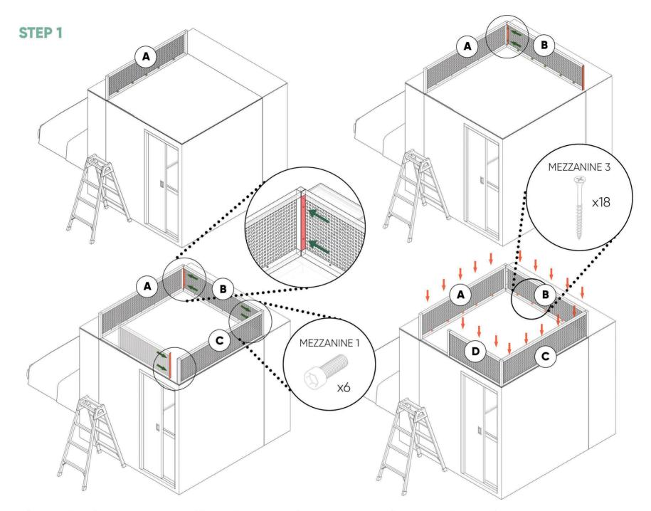
• Connect the elements on the top of the bathroom module using the screws (Mezzanine "1" and "3") according to the drawings.
