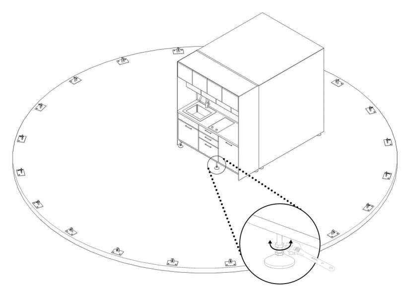
• Level the module using the adjustable feet so that it aligns with the bathroom module.
