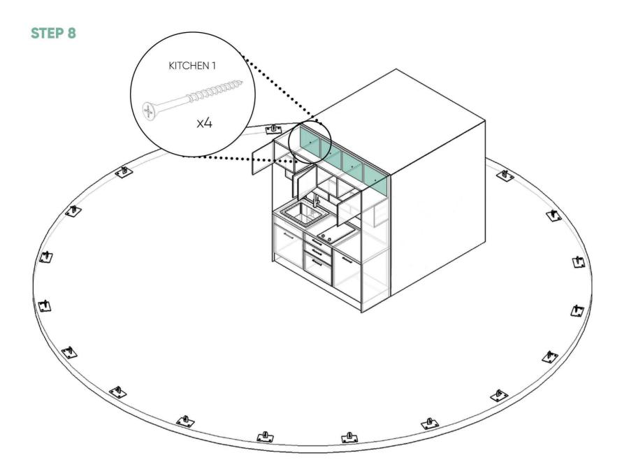
• Open the upper left cupboard and screw the screw through the back of the cupboard to connect the kitchen module with the bathroom module. Repeat the same for the rest of the cabinets.
